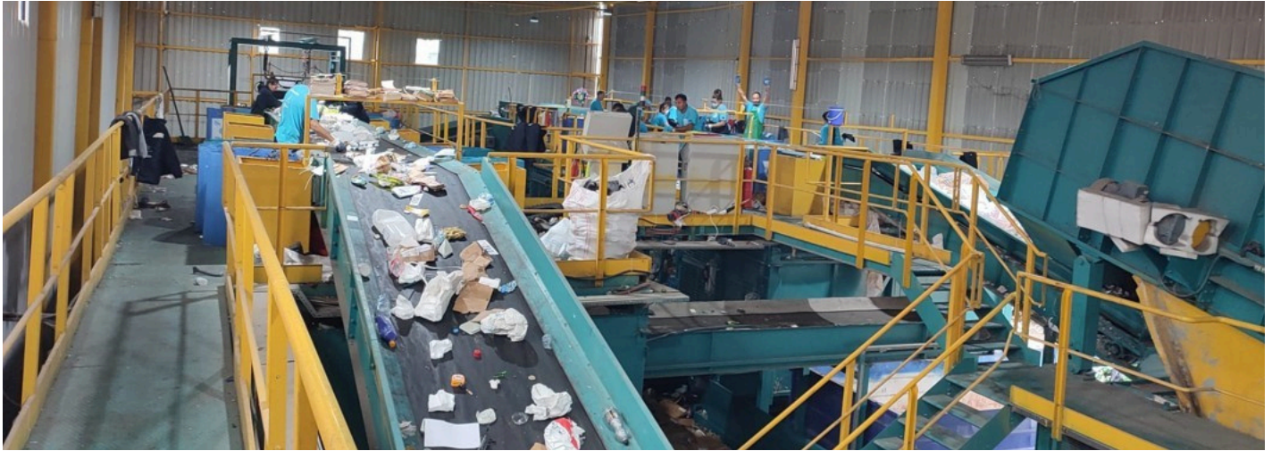
Waste segregation conveyor line in the sorting facility
