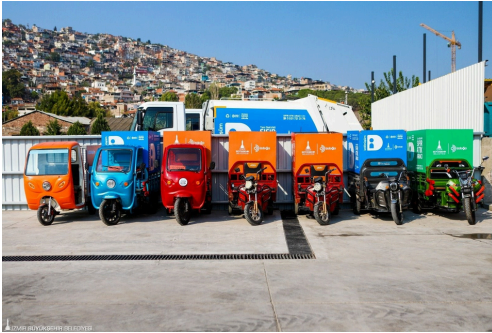
Customised vehicles outfitted with electric motorcycles are used to collect household waste
