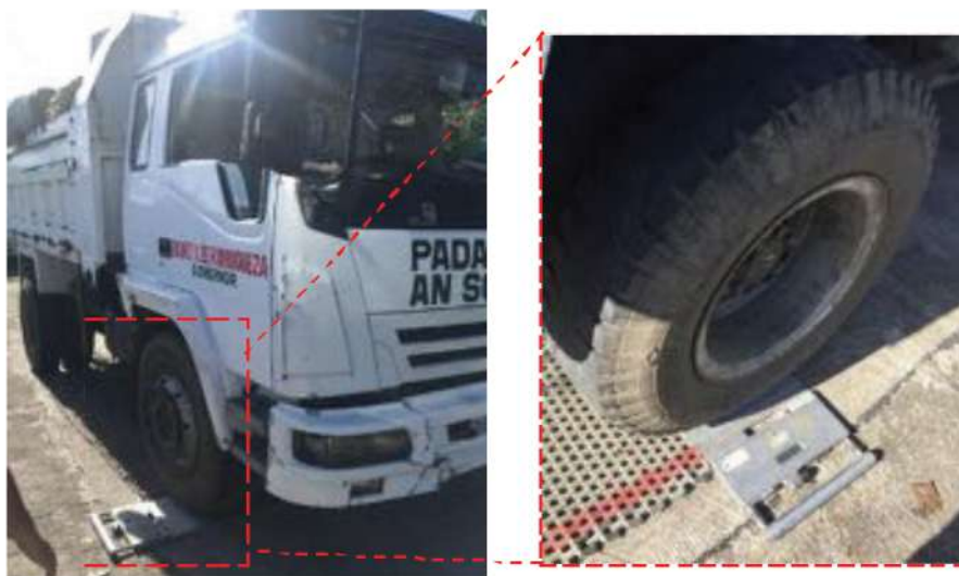
Figure 10. Weighing of Incoming Trucks using Weigh Pads
