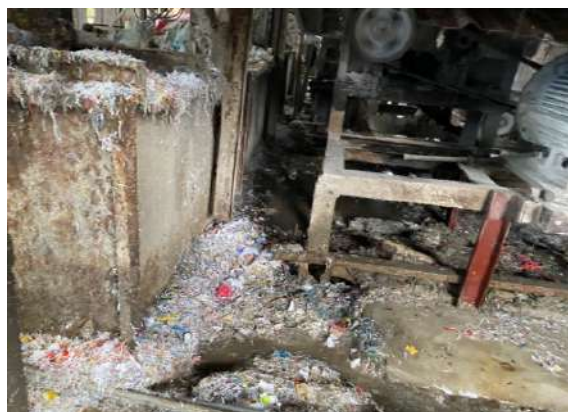
Figure 8.6. Plastic Losses During the Shredding and Flaking Process of Mechanical Recycling
